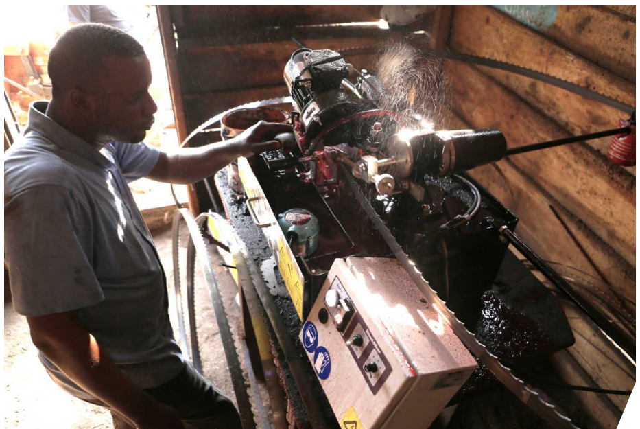
Wood-Mizer's blade maintenance machines make it easy for sawmillers to save money by sharpening and setting their own blades.
