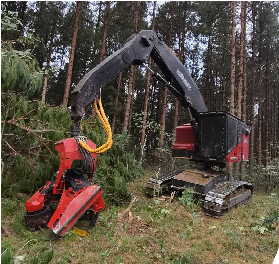
The TimberPro 725D and SP 761LF combination is proving to be an ideal solution for Mkhoba Forestry's steep slope harvesting operations.
