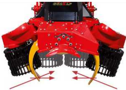
The proportionally angled feeder rollers of the SP head lessens friction.
