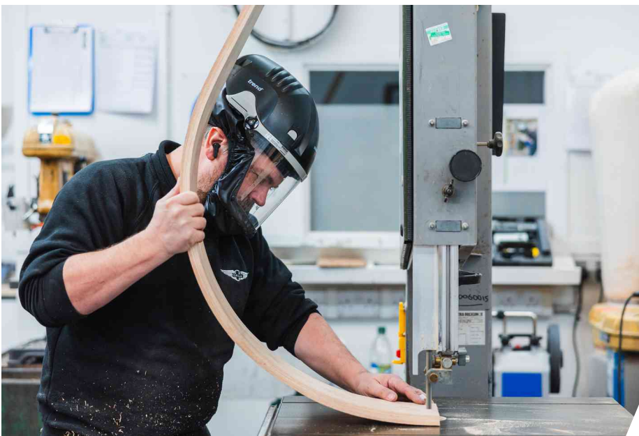
The ash timber body frame of Morgan cars are hand made by artisan coach builders. Pic credit Morgan Motor Cars.
