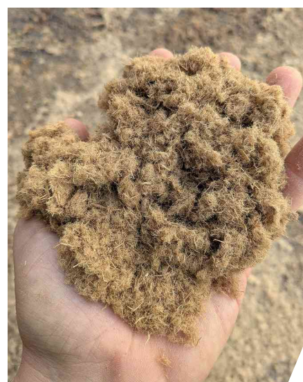
Fibres from waste fibreboard material recycled at Unilin's new Dieffenbacher Fiber2Fiber plant.
