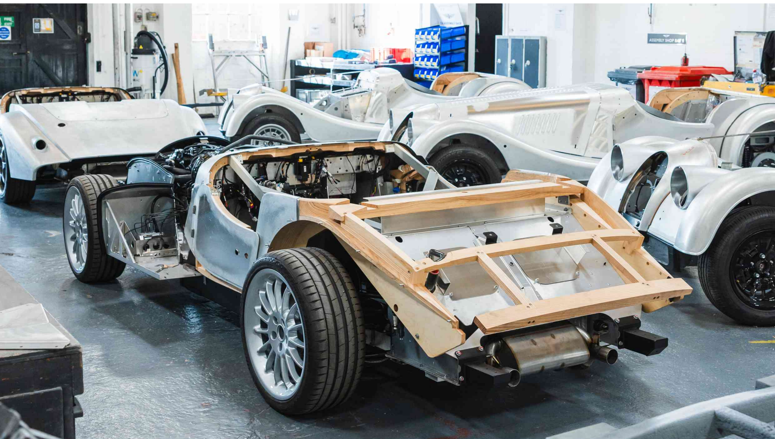
The aluminium body work is attached to the wooden frame in the Morgan factory. Pic credit Morgan Motor Company.
