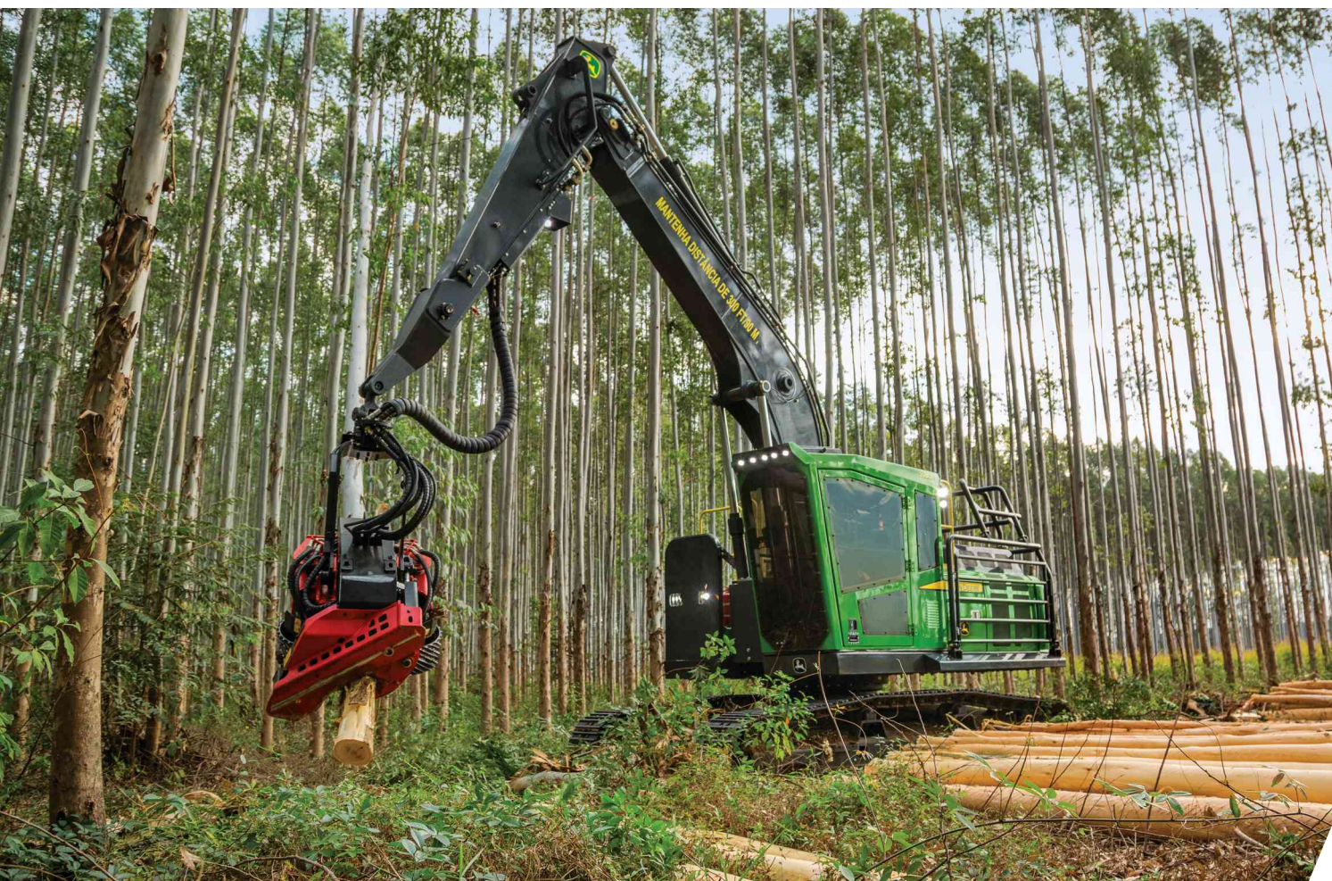
Safety is a priority and the top of the line cab is ROPS, FOPS and OPS certified.
