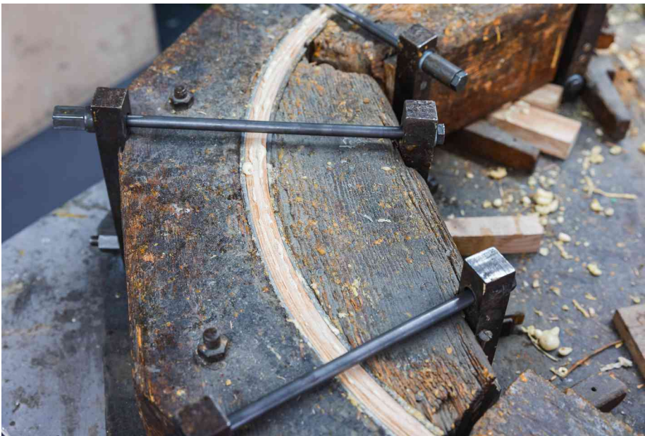
Steam bending a wheel arch. Pic credit Morgan Motor Company.
