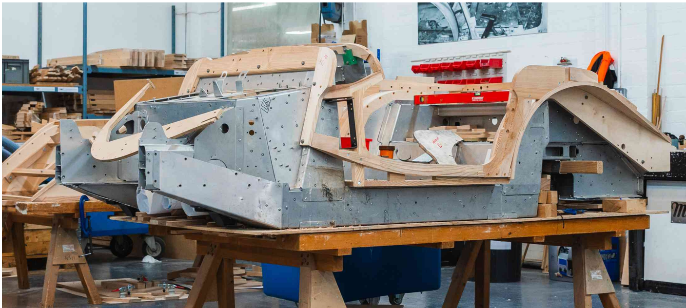
A Morgan Plus Six Model body takes shape. Pic credit Morgan Motor Cars.
