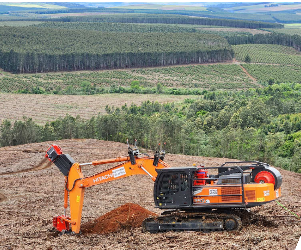
Cintasign forestry harvesting contractors has deployed a Hitachi 350 excavator fitted with the URUS TL3021 for steep-slope logging in KZN.
