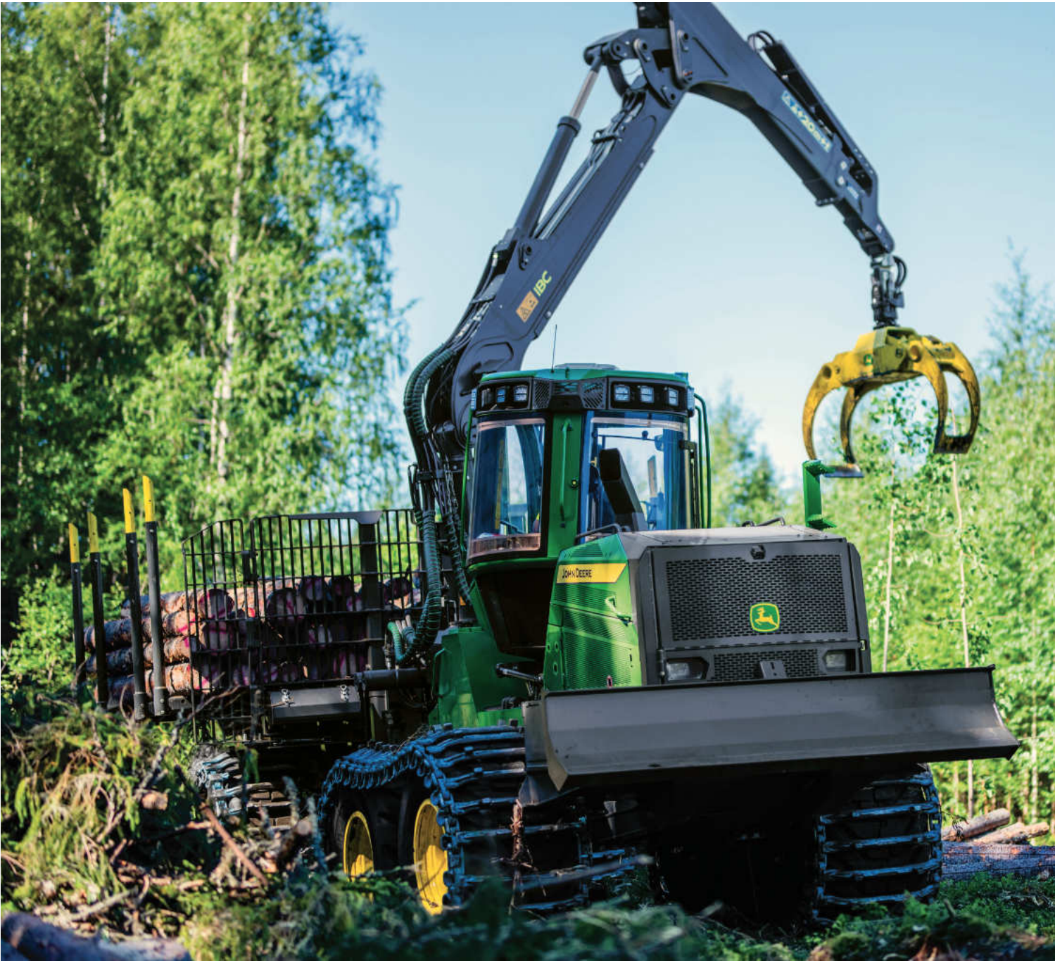
The 2010H has larger fluid tanks and improved diagnostics to optimise uptime.
