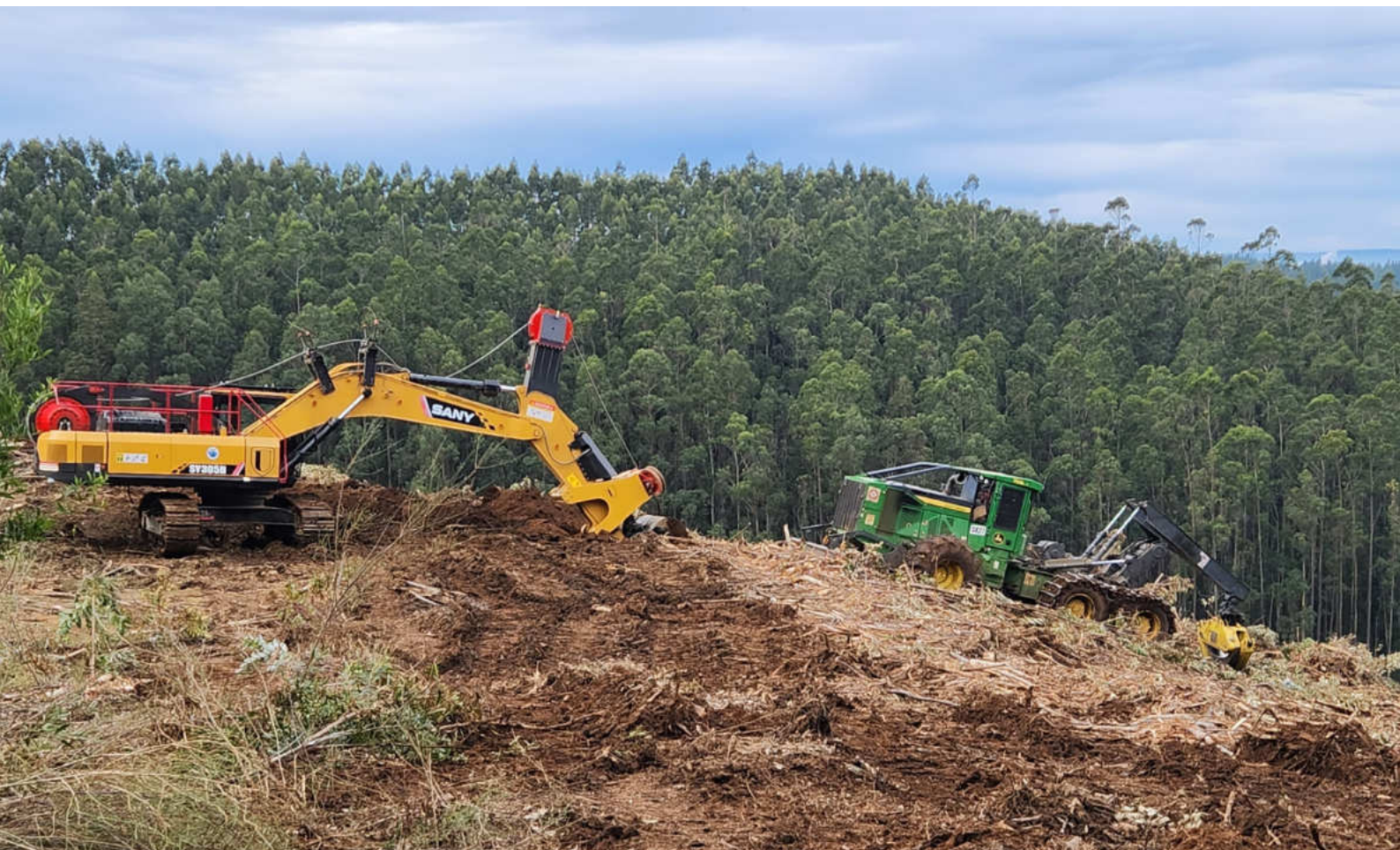
The Sany-URUS combo winch assisting a John Deere harvester.
