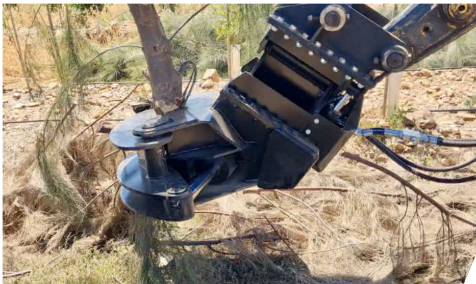
The Badger Bioshear cuts trees up to 250mm in diameter.
