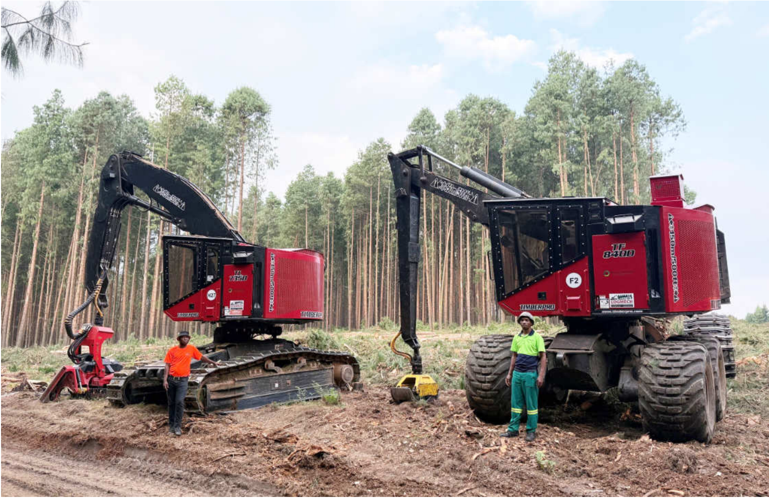
The TimberPro harvester fitted with an SP head and the TimberPro Forwarder are a purpose-matched harvesting team.
