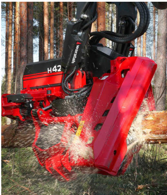
The heavy duty Waratah H427 harvester head.
