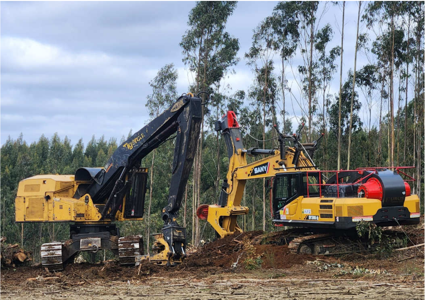
The URUS TL3021 mounted on a Sany excavator winch assisting a TCi Harvester.
