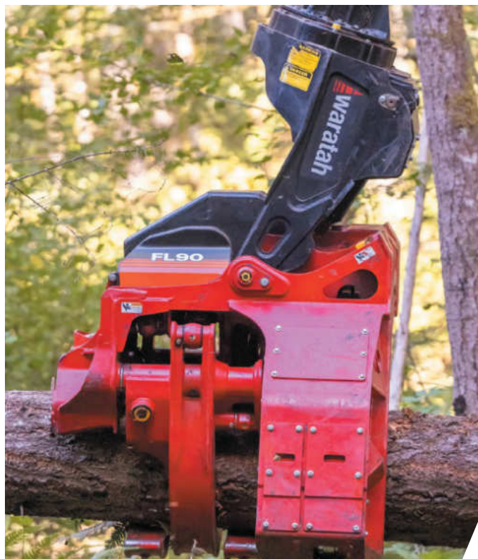
The Waratah FL90 directional felling head.
