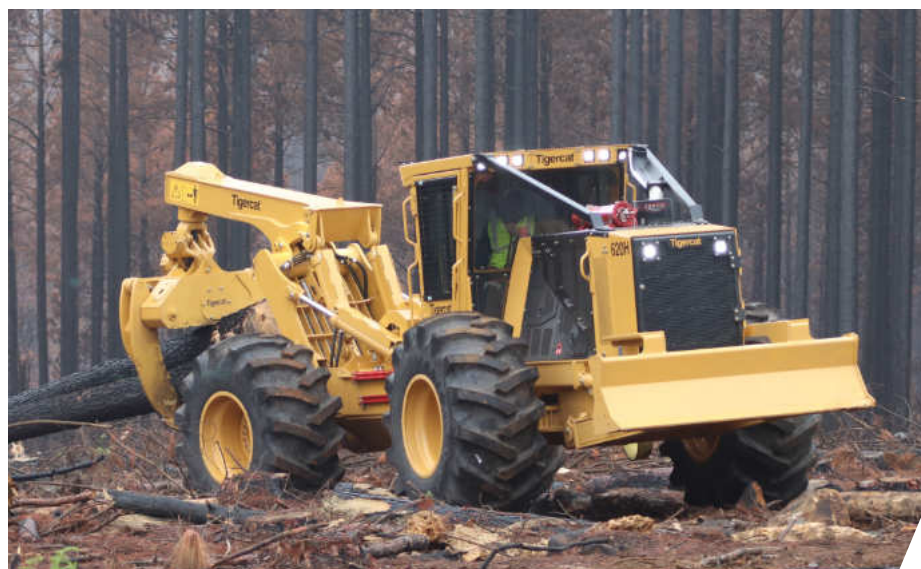
The high capacity TCi 620H four-wheel drive grapple skidder in action.
