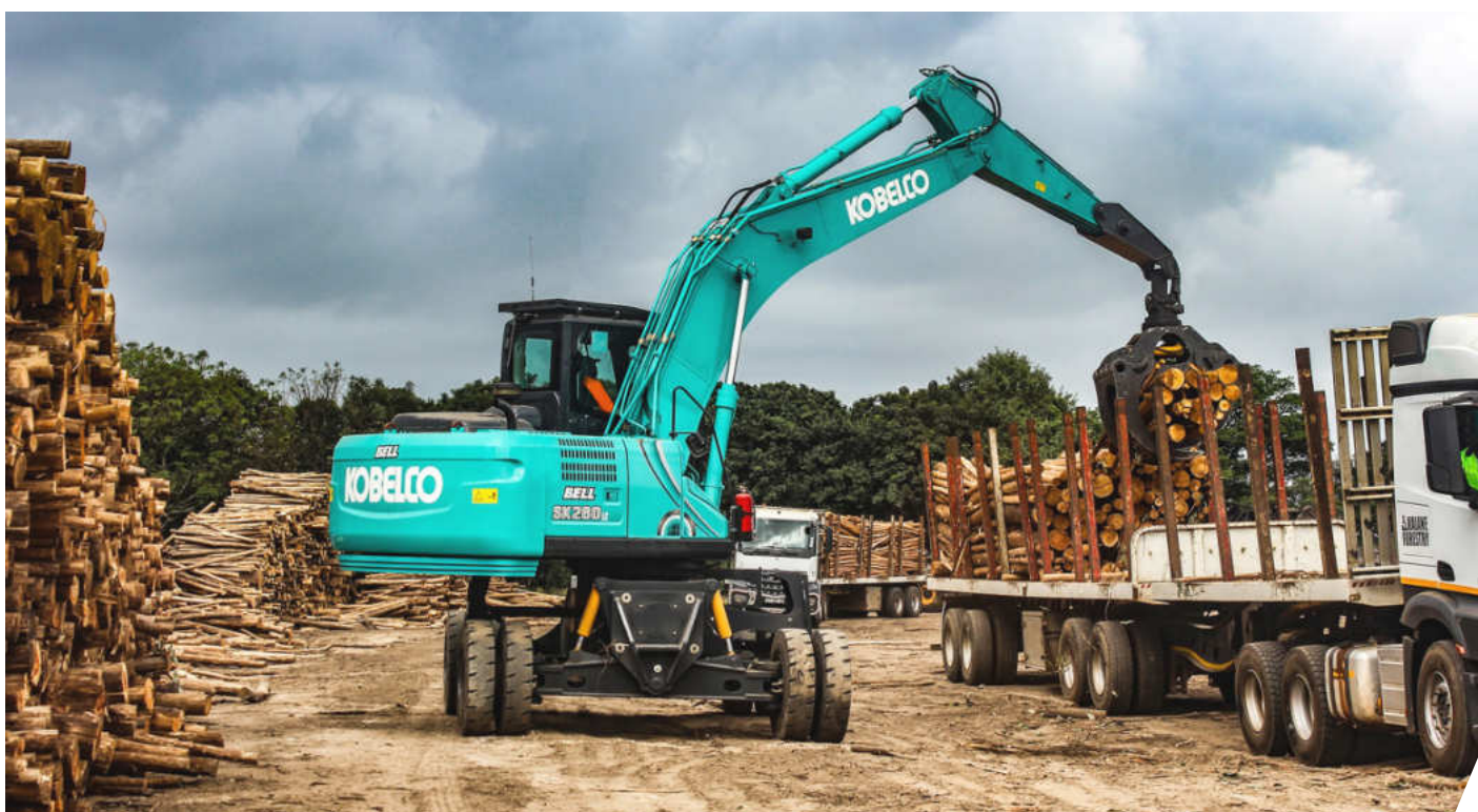
Bell supplied the Kobelco SK260LC-10 excavator fitted with a MT1000 timber grab.
