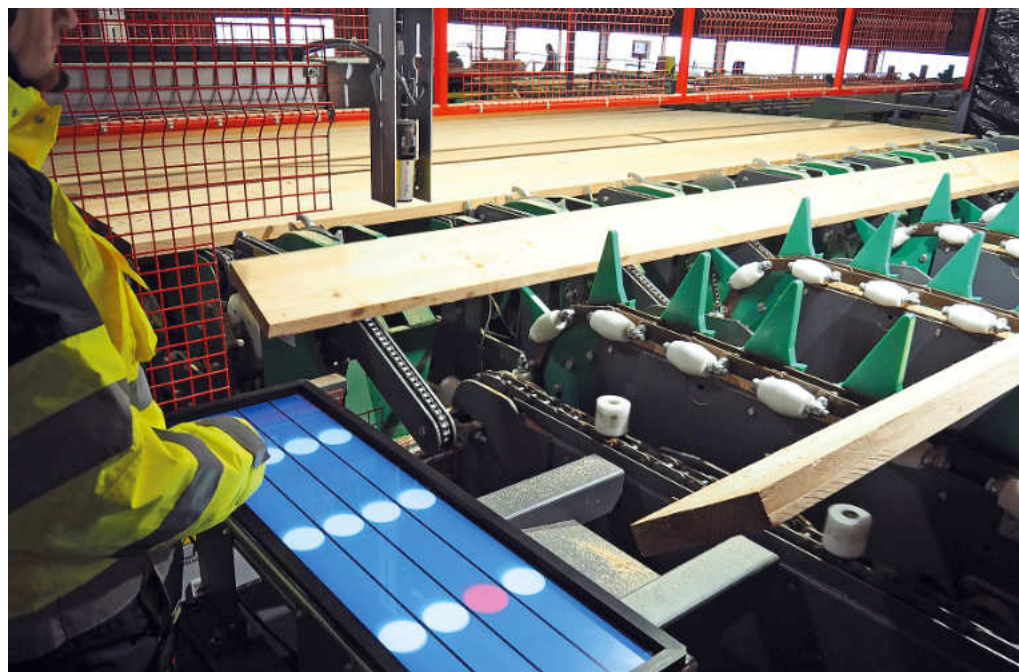
An employee inspects both sides of the timber using the assessment chain conveyor and enters the quality on the touchscreen (Pic by Holzkurier).
