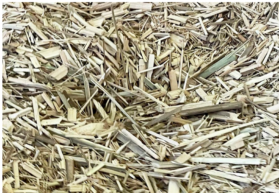
Shredded palm fronds will be used to produce HDF and MDF boards in Egypt.
