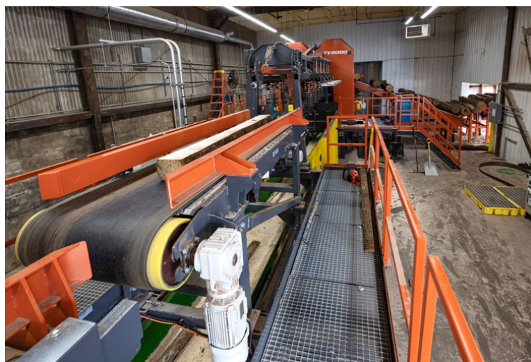
The belt conveyor centering table at Nelson Wood Shims.
