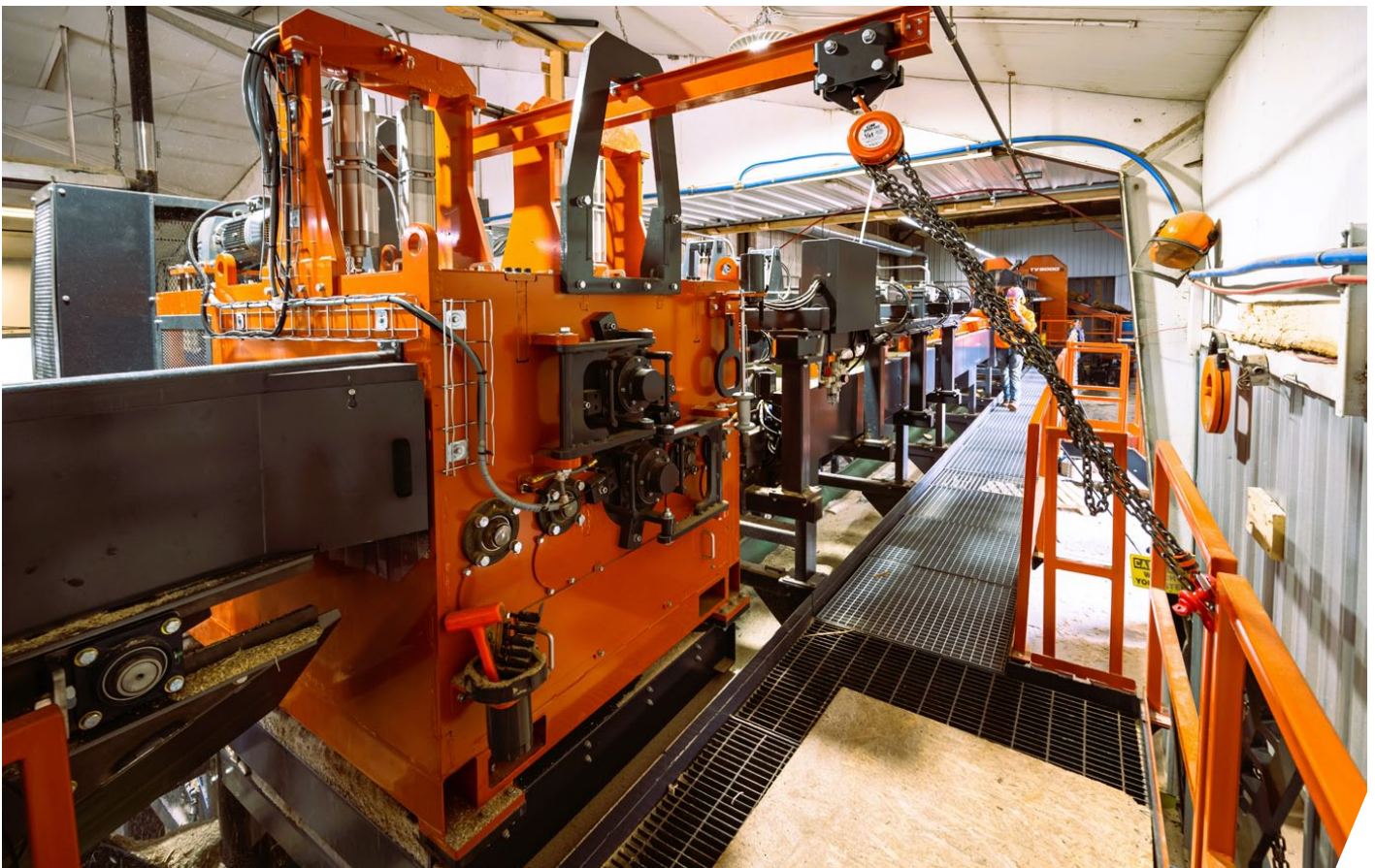
The Wood-Mizer heavy-duty TV6000 Twin Vertical saw prepares the cant for the multi-rip saw.
