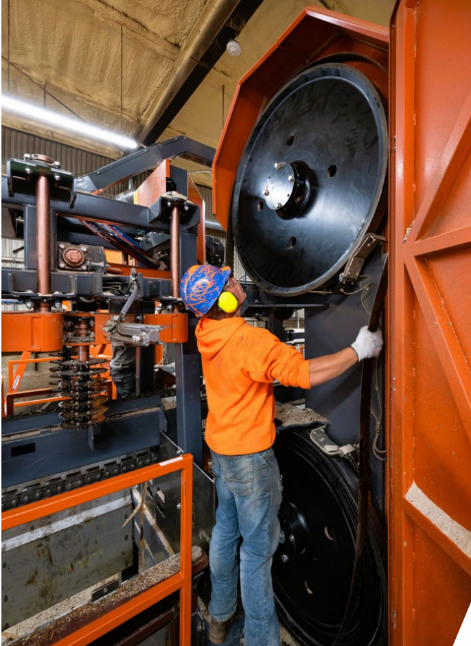
An operator changing a bandsaw blade of the impressive TV6000 twin vertical breakdown saw.
