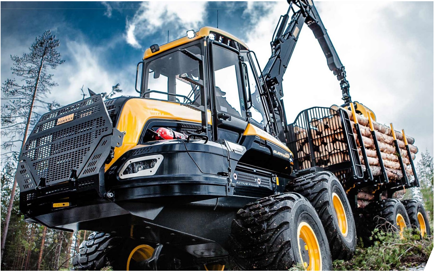
The Ponsse Elephant King with Active Crane is a formidable forwarder
